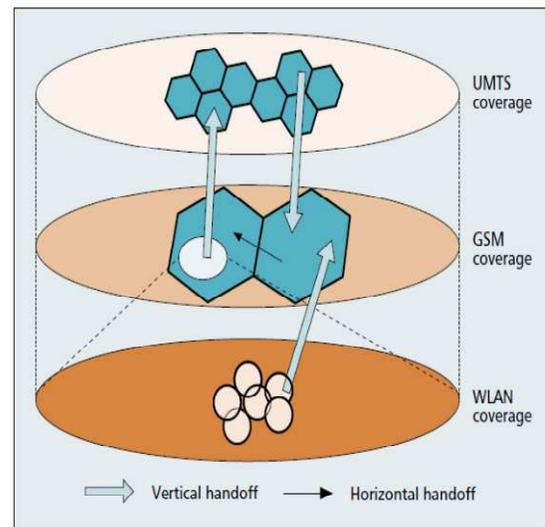
Fig 2. Vertical handoff and horizontal handoff of a mobile terminal [7]
