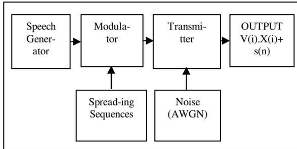
Fig. 1 Real Time System Model at Transmitter
