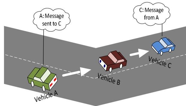
Fig. 3. Routing-based Communication
