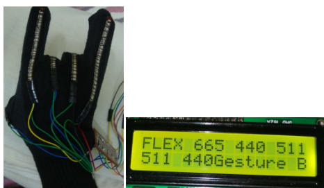
Fig. 8 Gesture-B made on glove & corresponding ADC outputs on LCD.
