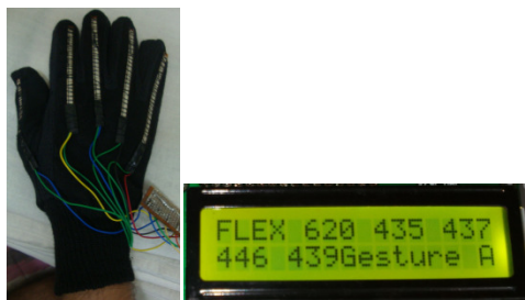
Fig. 7 Gesture-A made on glove & corresponding ADC outputs on LCD.
