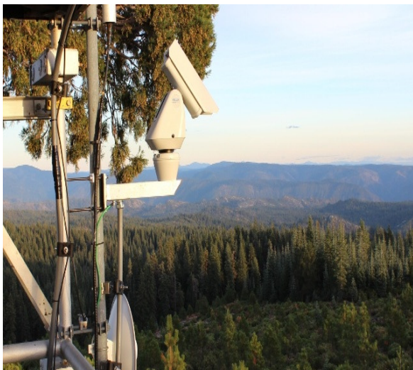
Fig. 1 Forest watch camera for detecting fire
