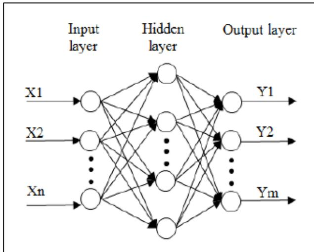
Fig 8. Structure of BP neural network
