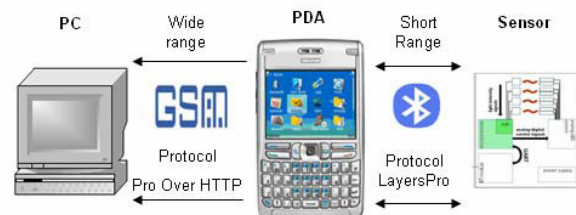
Fig 2: Application System Architecture
